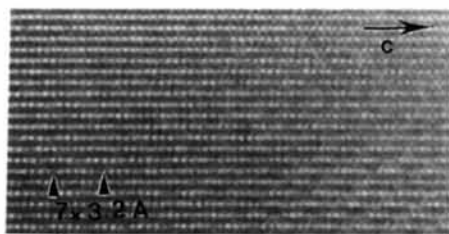
Fig. 10. High-resolution image, taken along the [1\bar{1}0] zone axis, showing a modulation of the sequence of intensities of bright and dark dots.
